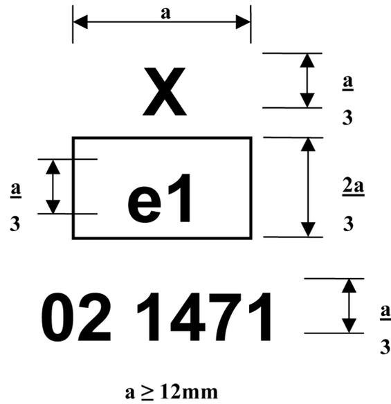
The device bearing the EC type-approval mark shown above is for a frontal protection system type-approved in Germany (e1) pursuant to this Regulation (02) under the base approval number 1471.
